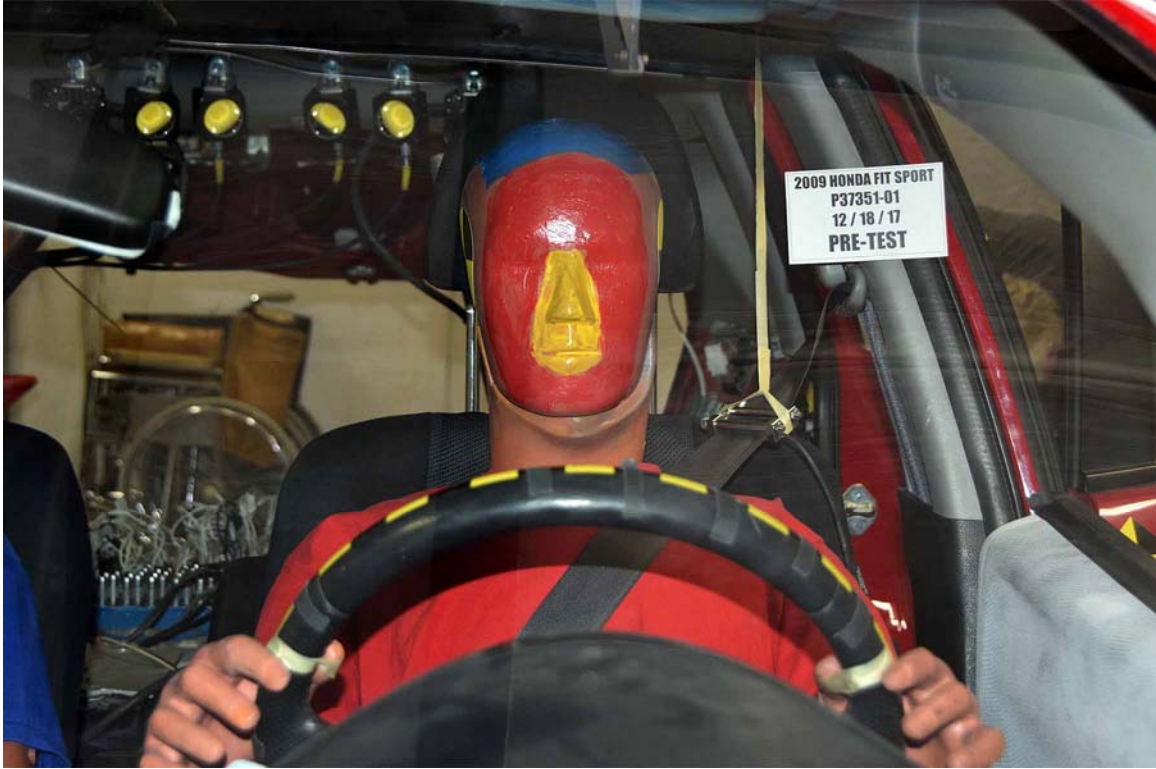
FIGURE 25. Pre-Test Front View of Driver Dummy
