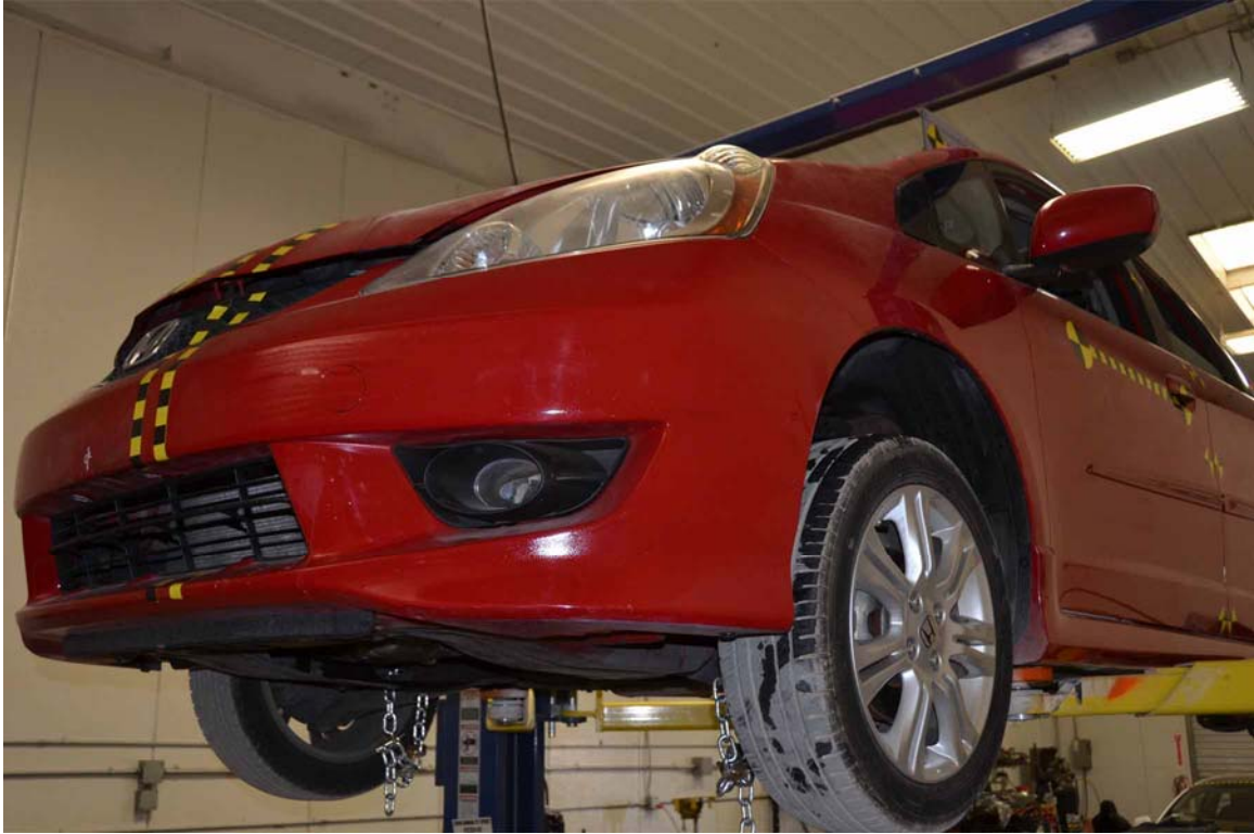
FIGURE 23. Pre-Test Vehicle Impact Area
