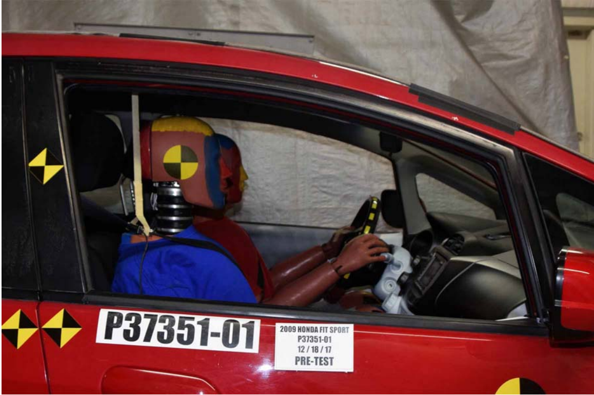
FIGURE 45. Pre-Test Side View of Passenger Dummy
