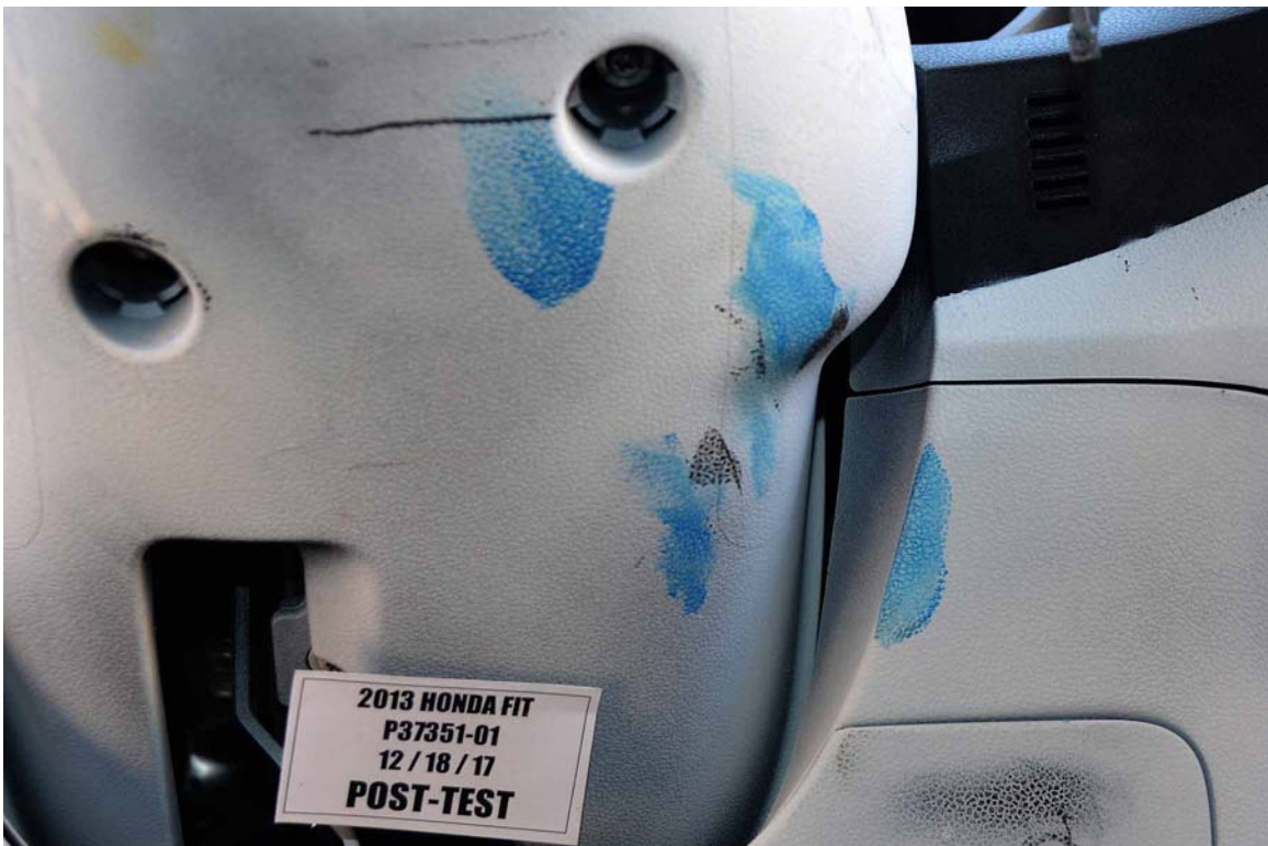
FIGURE 40. Post-Test Driver Dummy Contact with Steering Column
