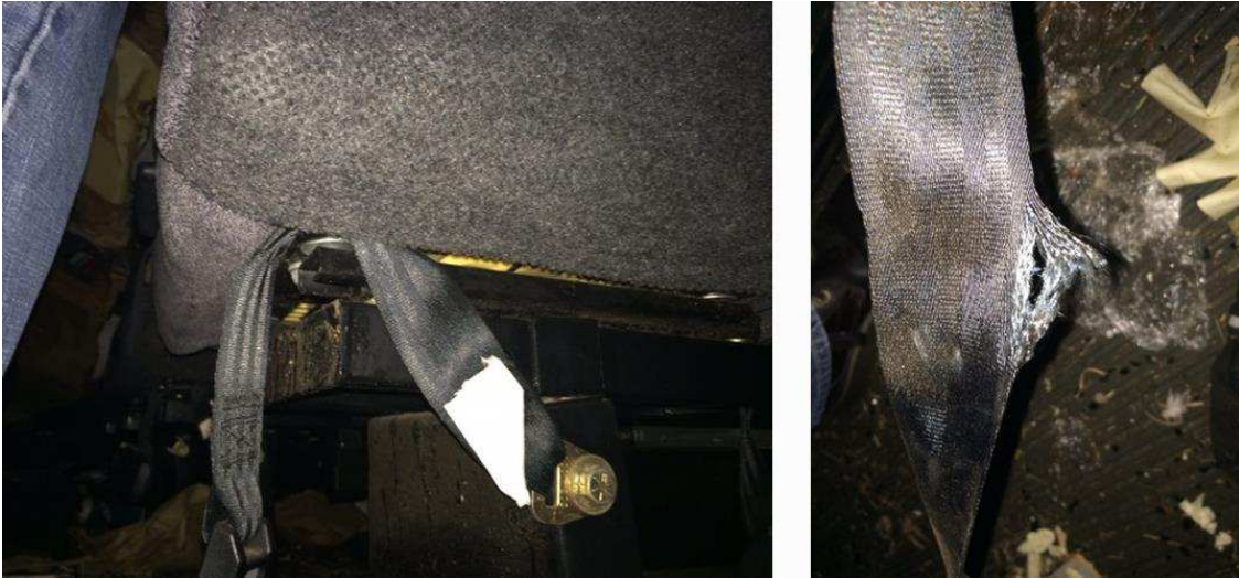
Figure 7. Seat belt webbing pinched above side-slide seat track (left) and torn seat belt webbing on side-slide seat (right).
