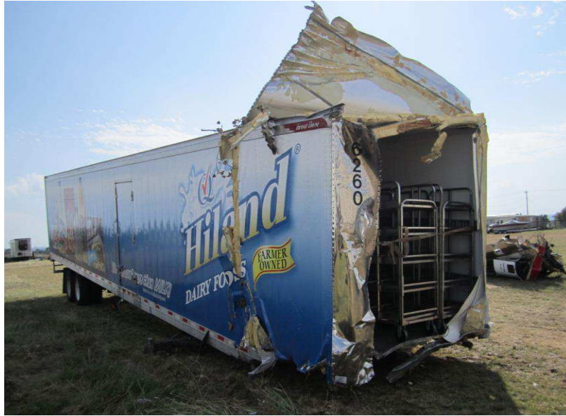
Figure 9. Semitrailer postcrash, showing damage to front end and roof.
