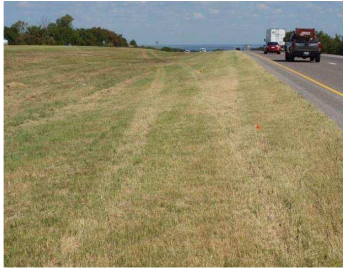
Figure 14. Tire marks alongside I-35 northbound, showing path followed by truck-tractor as it crossed 100-foot-wide median and entered southbound lanes.
