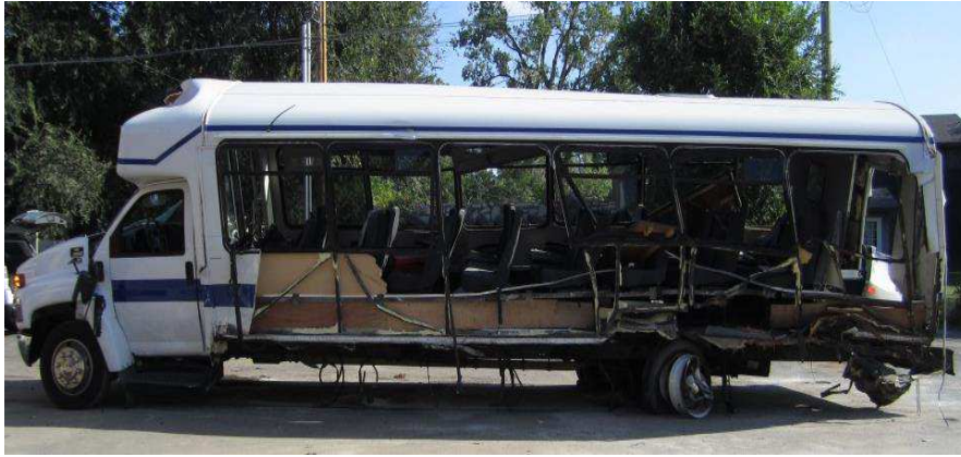
Figure 10. Driver side of bus postcrash, with all main windows broken out and outer body panels missing.
