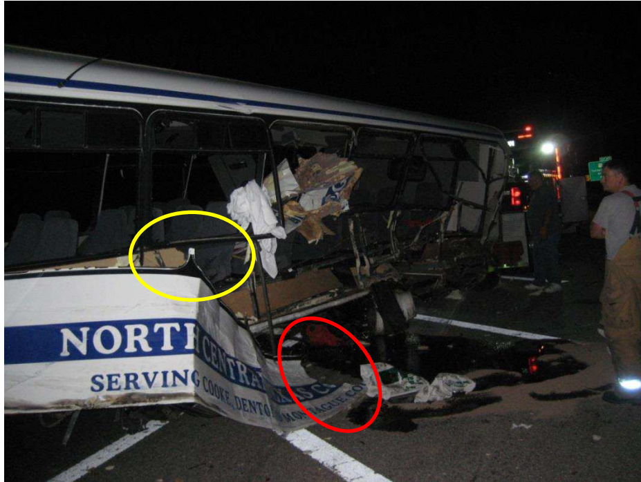
Figure 13. Damage to sidewall support structures on driver side of bus, with yellow circle highlighting broken joint and red circle highlighting panel tearing. (Source: Oklahoma Highway Patrol)
