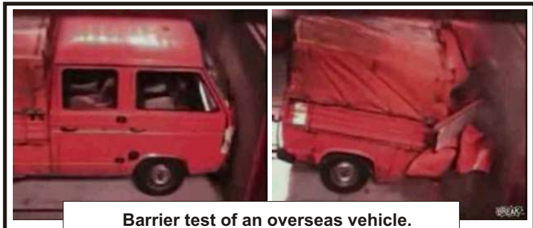
Barrier test of an overseas vehicle. The passenger compartment is completely destroyed.
