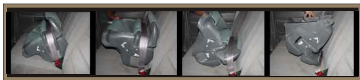
Booster seat rolls out from under belt
