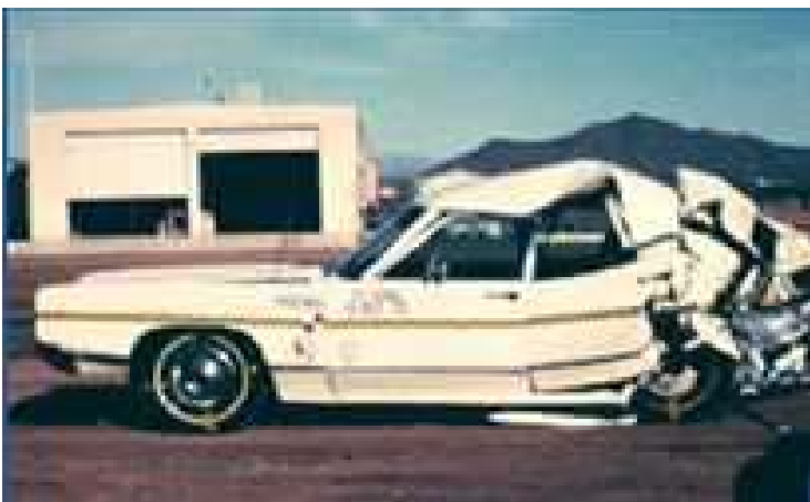
Fuel tank in front of axle - no leakage
