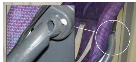
Fractured tray shield
