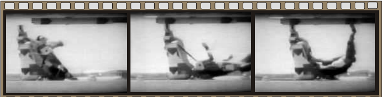
Frontal Impact - Shoulder Belt Only Sequence
