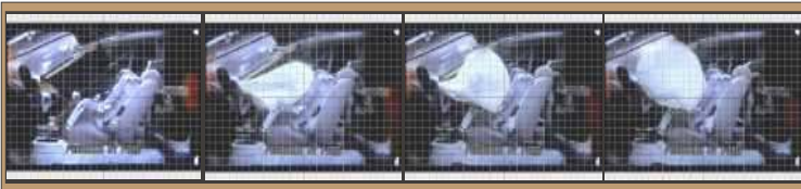
Airbag Deployment Sequence - Forward Facing Child Seat
