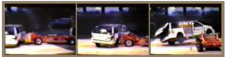
Liftgate Opens - Side Impact
