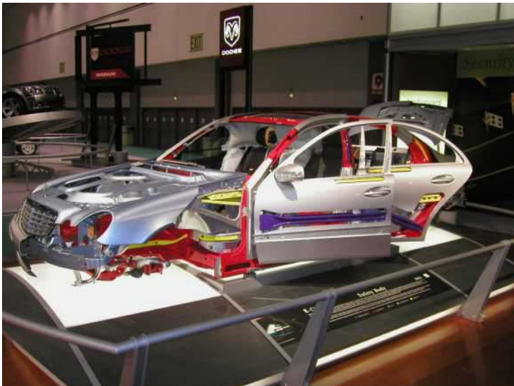
Energy Channeling and Load Bearing Structures
